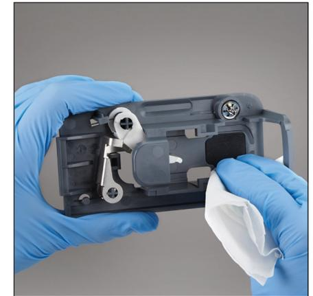
4. Clean the **entire** base using a lint-free wipe or cotton swab dampened with 70% isopropyl alcohol, mild liquid soap and water, or a 10% bleach solution.
