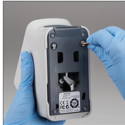
2. On the bottom of a powered-off analyzer, use a flat-tip screw driver or coin to turn the 2 silver fasteners counterclockwise a quarter turn.
