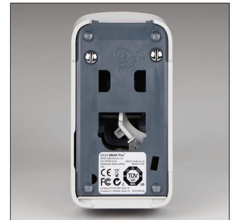
8. Ensure the base and silver fasteners are flush with the analyzer and locked into place. **Not locking the base and fasteners properly can impact analyzer performance.**
