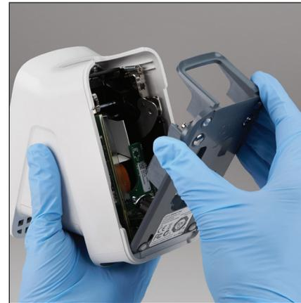
3. Remove the base from the analyzer.
